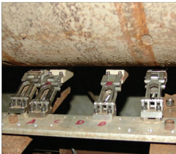
Fig. 5: Eddy current sensors in rotary test rig setup
