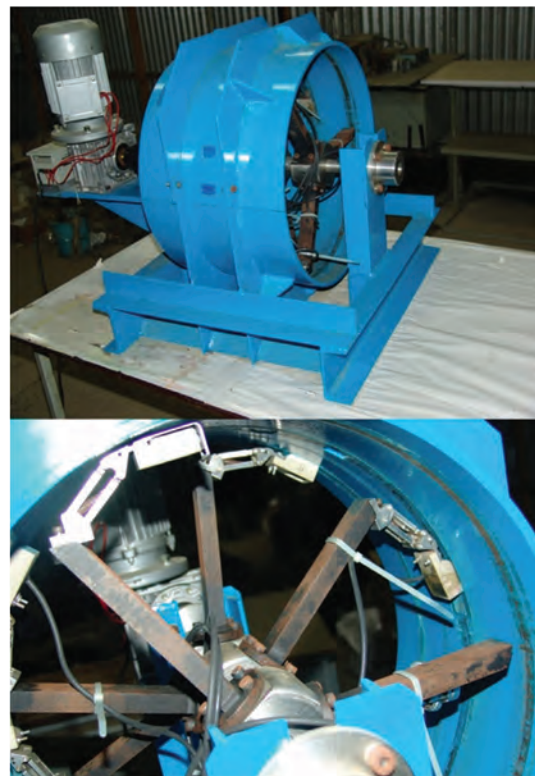
Fig. 7: Dynamic test setup for wear and endurance verification
