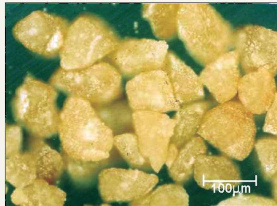
Fig. 2: Particle morphology of sintered  $GdAlO_3$  granules
