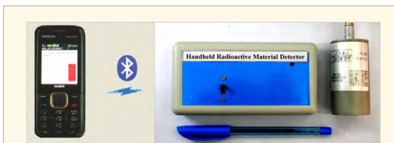
Fig. 1: Handheld Tele Radionuclide Detector with controlling mobile phone.
