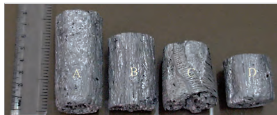
Fig. 5: Aluminium foam samples used for compression testing (Front view)
