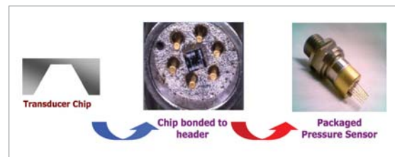
Fig.13: Process Route from sensing diaphragm to packaged pressure sensor
