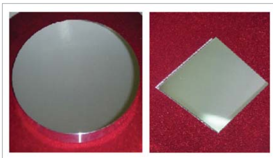
Fig. 2 : Solid circular and square honeycomb Al-alloy mirrors machined by DTM
