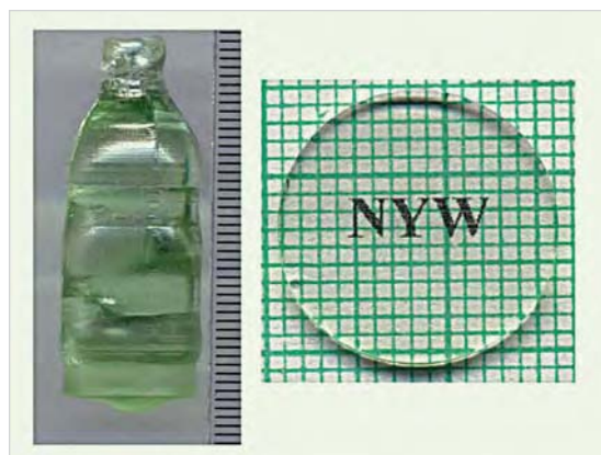
Fig. 13: Photograph of as-grown single crystal of \text{NaY}(\text{WO}_4)_2 (left) and polished disc.
