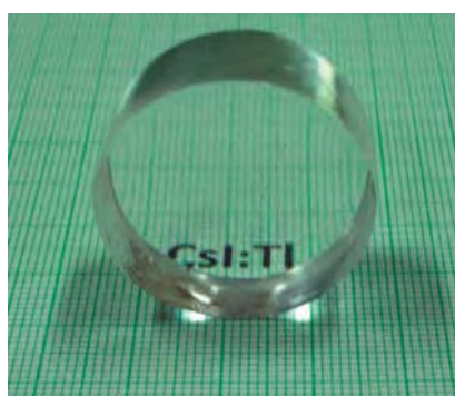
Fig. 3: Photograph of a polished single crystal of CsI:Tl grown by gradient freeze technique in carbon coated crucible.
