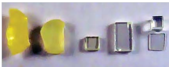
Fig. 6: Color transformation from yellow to transparent in PbWO_4 crystals.
