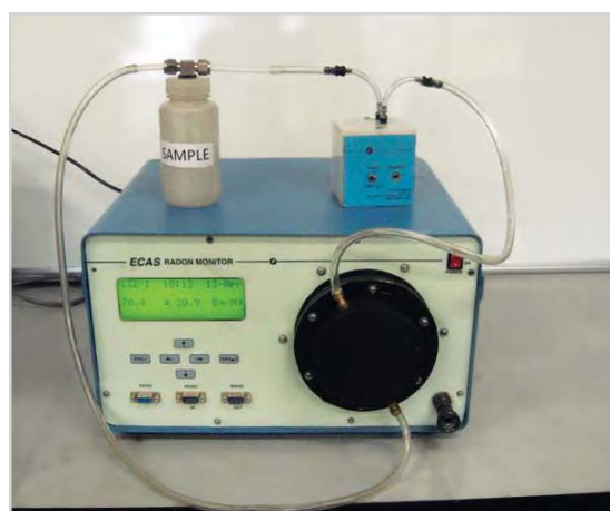
Fig. 10: Measurement of radon emission from a cement sample
