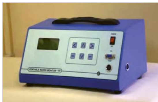
Fig. 1b: Photograph of Portable Radon Monitor (SRM)
