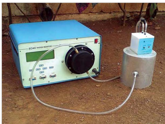
Fig. 9: Measurement of radon emission from soil
