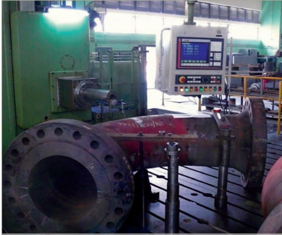
Fig. 9: CNC machining of notches on 600 NB Elbow specimens
