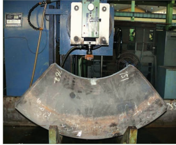
Fig.10: EDM machining of notches on 500 NB Elbow specimen
