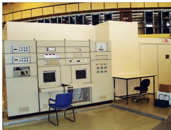
Fig. 4(b): Photograph of the control consol and shielding hutch of the dispersive EXAFS beamline
