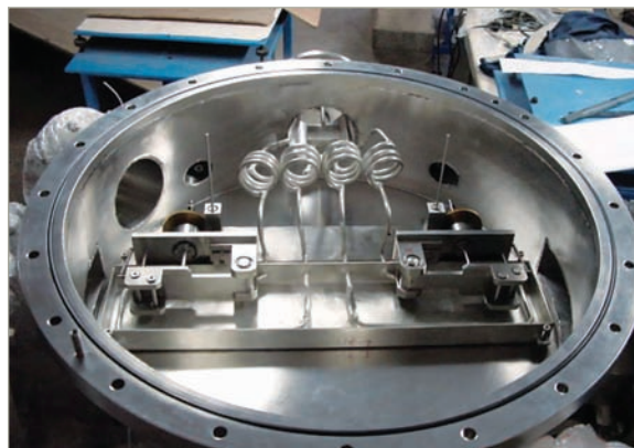
Fig. 4(d): Photograph of the crystal bender assembly developed in collaboration with CDM, BARC
