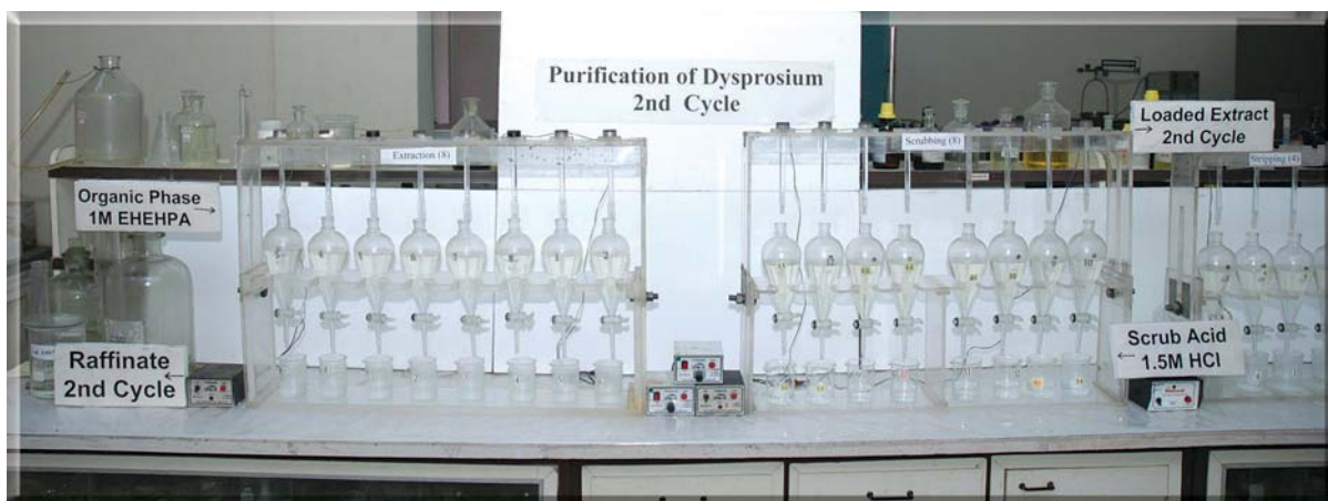
Fig. 6 : Counter-current lab set-up with specialized motors for purification of Dysprosium in cycle-2
