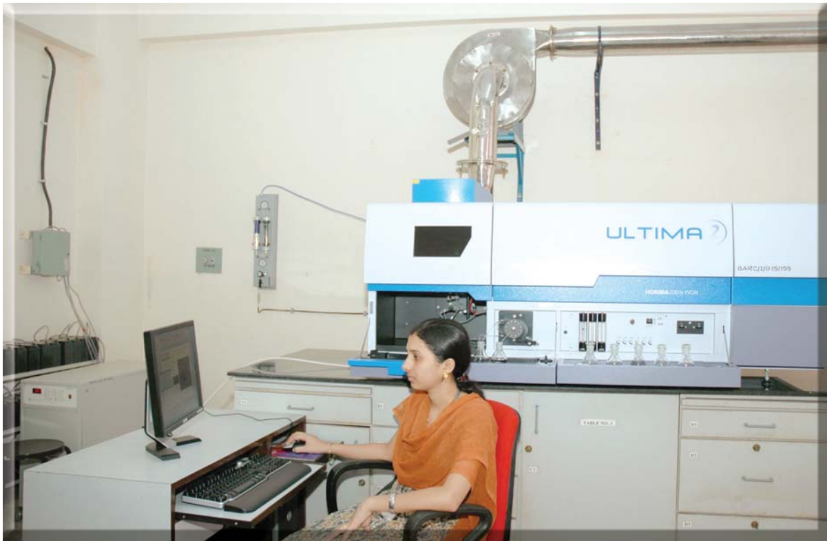
Fig. 11 : A high resolution ICP-AES installed at REDS
