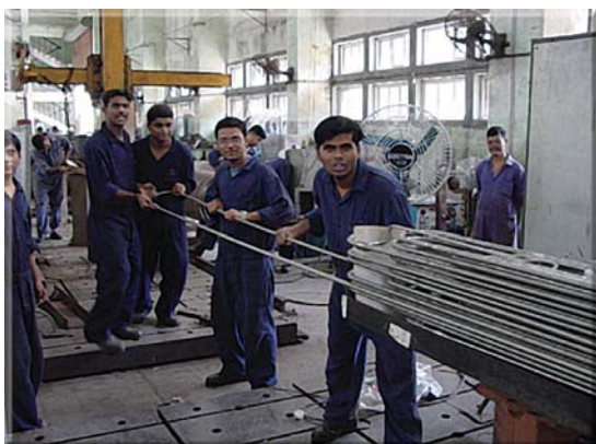
Fig. 6 : Insertion of U-tubes in the Tube Bundle
