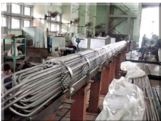
Fig. 7 : Tube Bundle final Assembly
