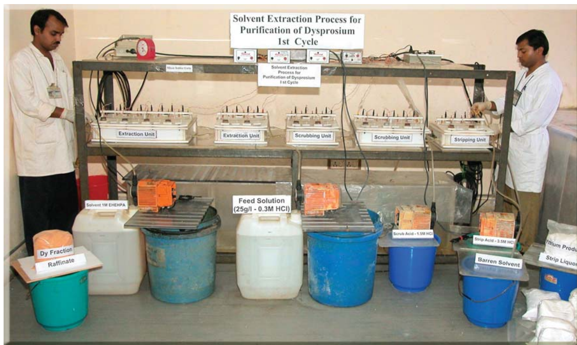
Fig. 3 : Mixer-settler cascade system for purification of Dysprosium cycle-1
