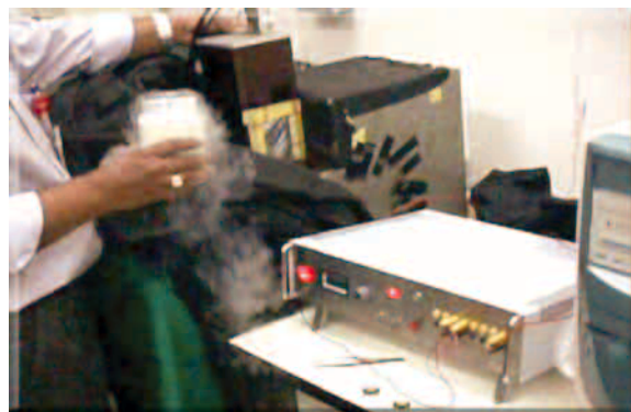
Fig.3b: Digital recording system interfacing thermoluminescence set-up
