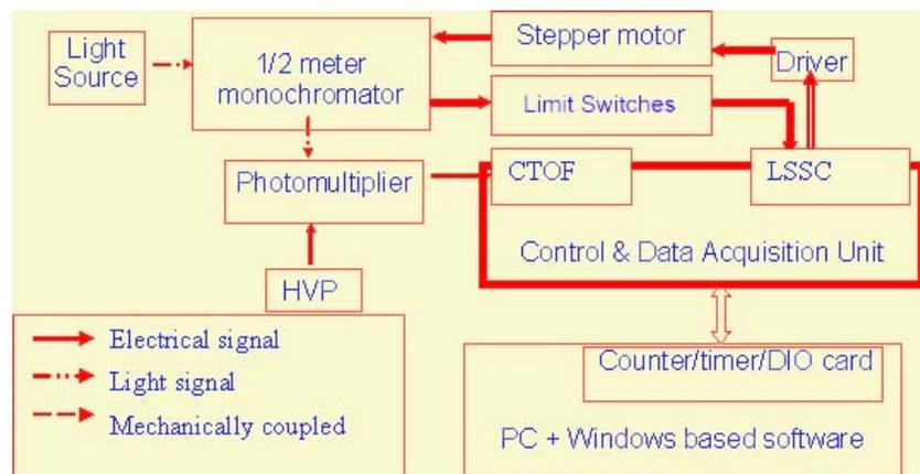
Fig. 3. Schematic block diagram of data acquisition system.
