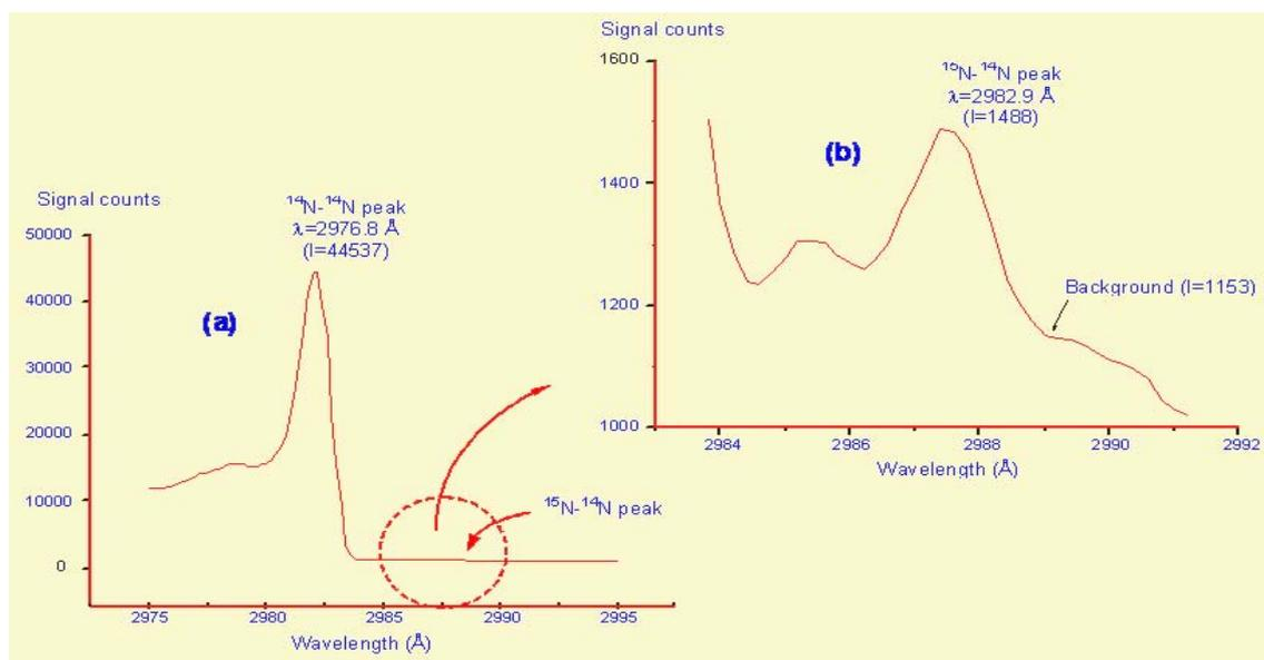
Fig. 5. Spectrum of nitrogen present in natural air recorded using the instrument. Plot (a) shows the peak of  $^{14}\text{N}-^{14}\text{N}$  molecule and plot (b) shows the enlarged plot of  $^{14}\text{N}-^{15}\text{N}$  peak.
