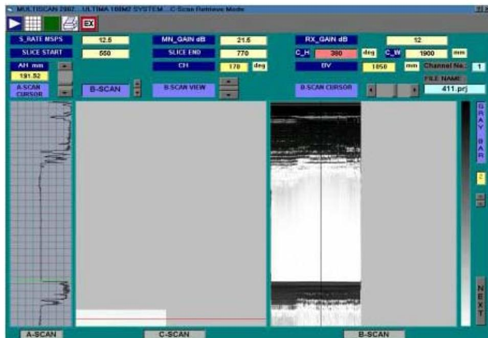
Fig. 5 Retrieved C-scan image of End Fitting forging using ULTIMA-100M4
