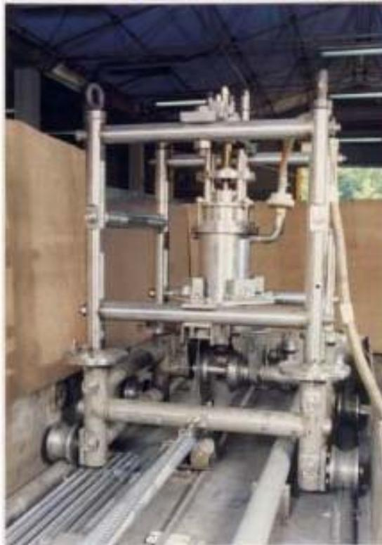
Fig.3 Buggy with cutting mechanism
