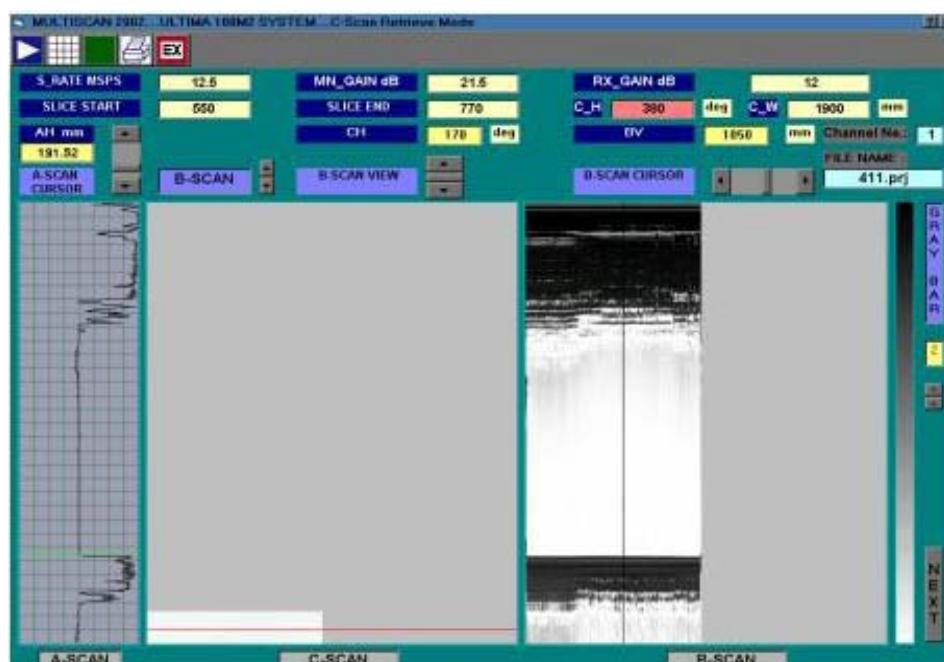
*Fig. 5. Retrieved C-scan image of End Fitting forging using UII TIMA-100M4*
