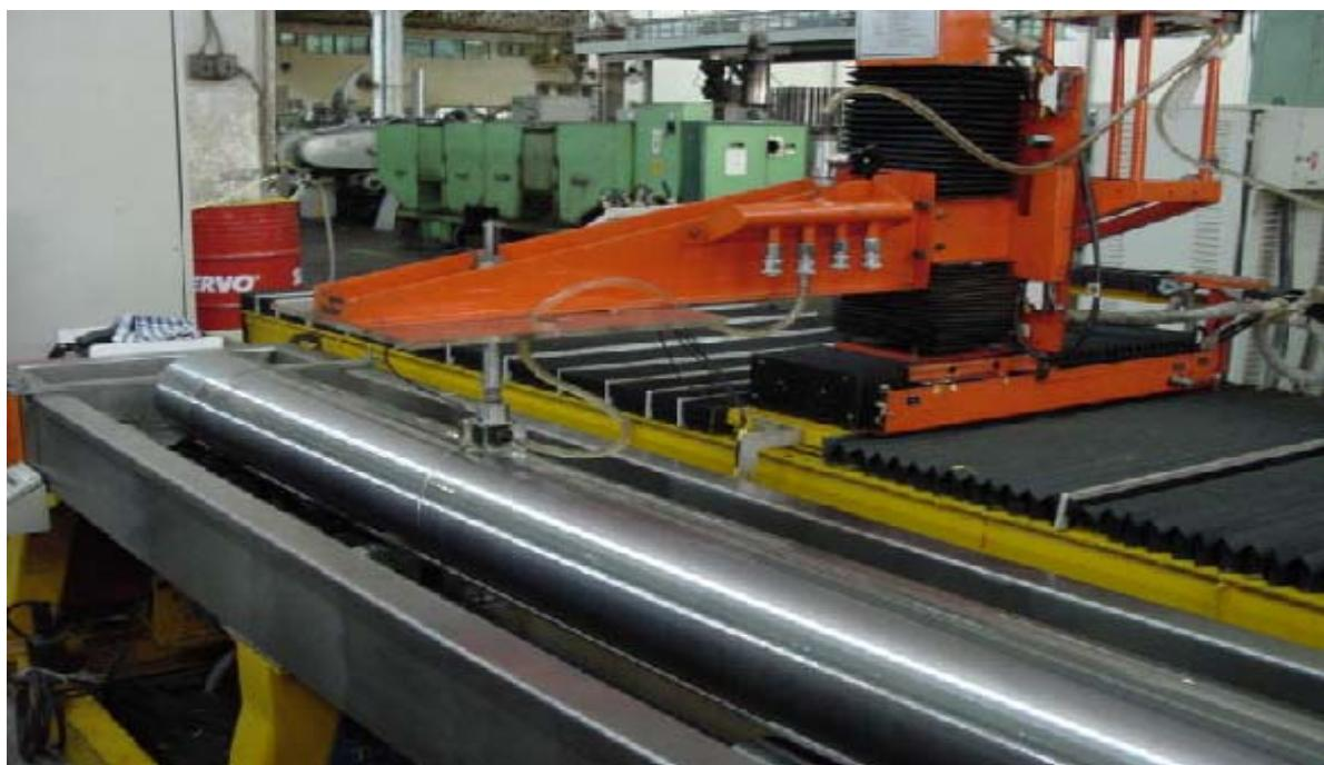
Fig. 6 Scanning of End Fitting forging by four-axis Automated Scanner in progress
