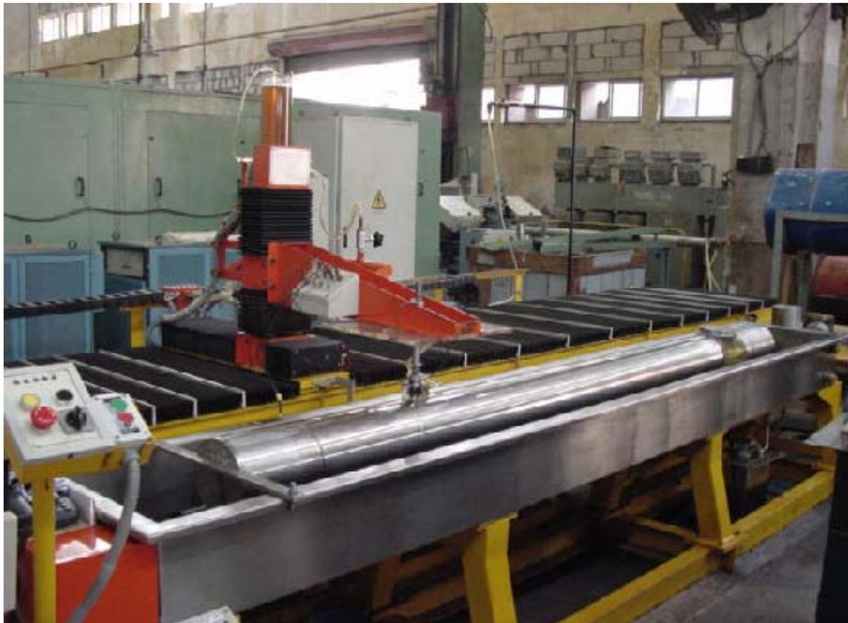
*Fig. 1 An overall view of four-axis Automated Scanner*
