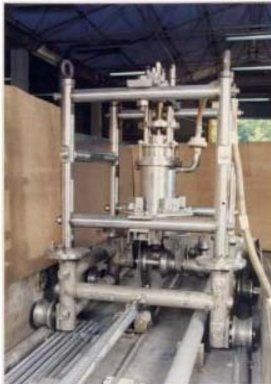
*Fig.3 Buggy with cutting mechanism*
