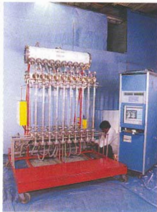
Experimental facility to study flow distribution in a natural circulation driven system
