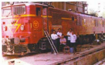
Plate 1. The electric locomotive, retrofitted with thyristor control system at ELW, Bhusawal
