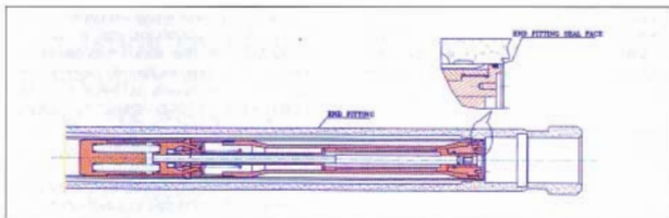
End fitting seal face is opened and ready for lapping
