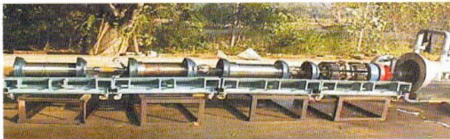
Fig 1 : Launching of IPIG at wet test loop at Faridabad.
