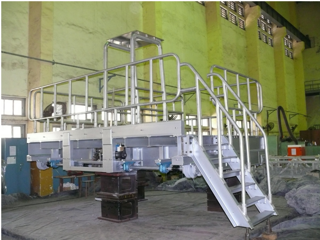
Fig: Automated Core Handling System for Upgraded Apsara Reactor
