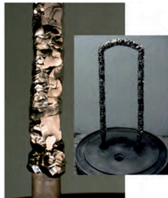
Fig. 3b: Zirconium crystal bar grown by iodide refining technique at BARC campus and the inset shows the crystal bar zirconium formed on U-shaped zirconium filament
