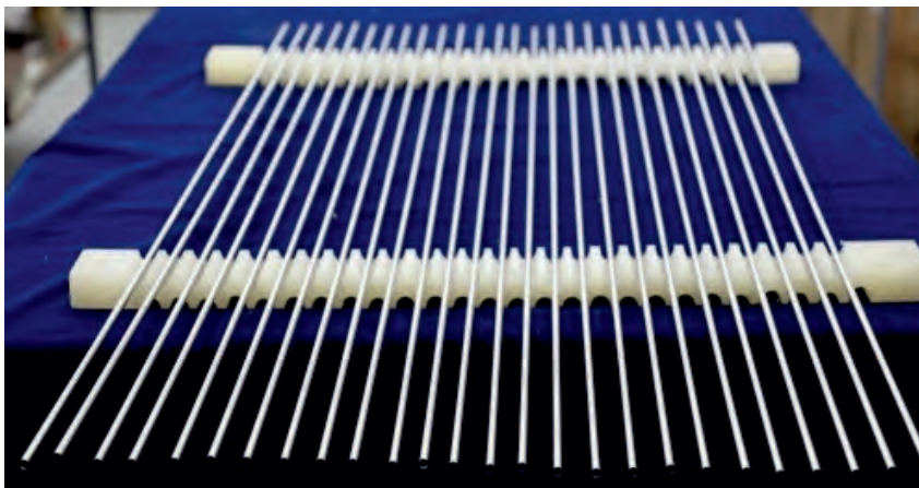
Fig.8: Typical picture of SuperNi 42 Tubes
