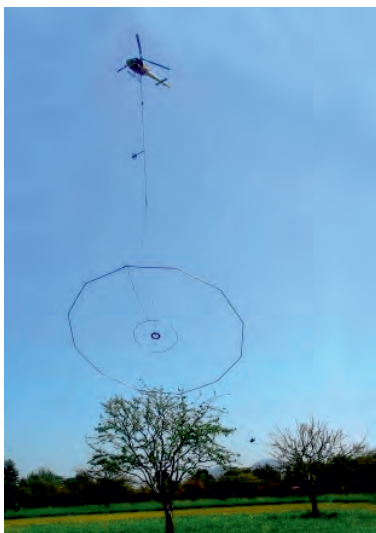
Fig. 3: Heliborne Geophysical Surveys conducted by AMD
