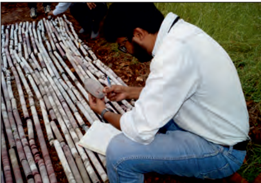
Fig. 6: On-site drill core examination by AMD geologist
