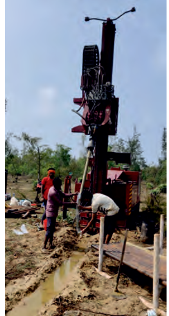
Fig. 11: Sonic Drilling in Beach sands of Brahmagiri area, Puri district, Odisha.
