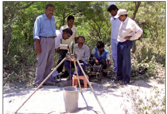
Fig. 7: Gamma ray logging of borehole
