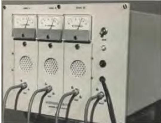
**Fig. 3: Three channel hydrogen monitor**
