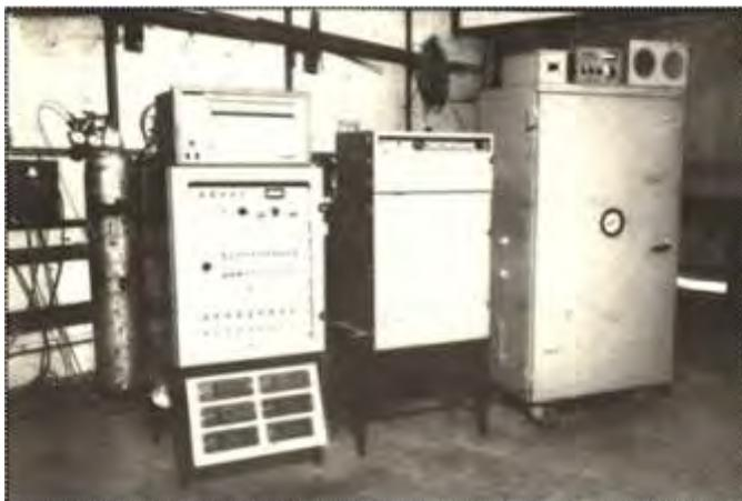
**Fig. 4: MAPS cover gas analyzer developed at Chemistry Group, BARC**
