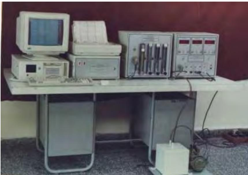
**Fig. 7: PC based multi stream hydrogen monitor for H<sub>2</sub> mitigation experiments**
