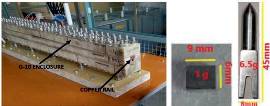
Figure 35.9(a). EM Rail-gun structure, (b). 1 g armature and (c). 6.5 g armature.
