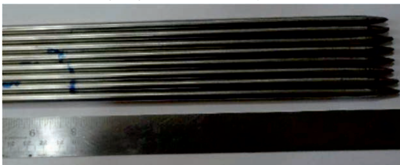
Figure 30.1. Indicative MP Welded fuel clad to end plug samples (OD 6.6 x 0.45 mm thick).
