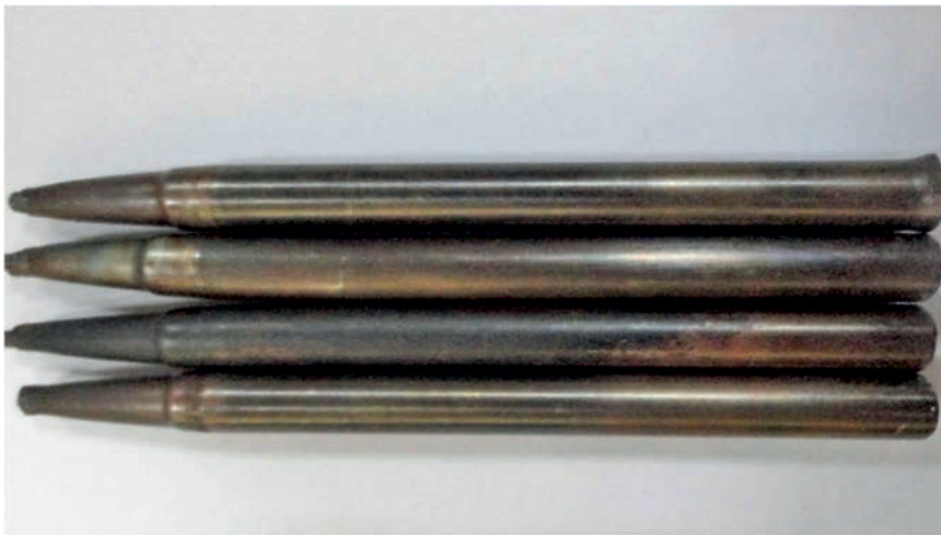
Figure 30.7. EM Welded samples after five thermal cycle (823K, 1800sec-300K, 1800sec) in air furnace.
