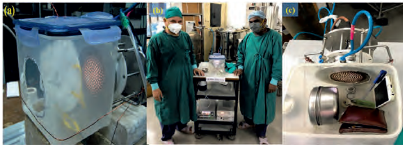
Figure 26.5: (a) Ongoing cold plasma treatment of N-95 mask, (b) typical cold plasma disinfection set-up, (c) Disinfection of personal belongings under cold plasma treatment.
