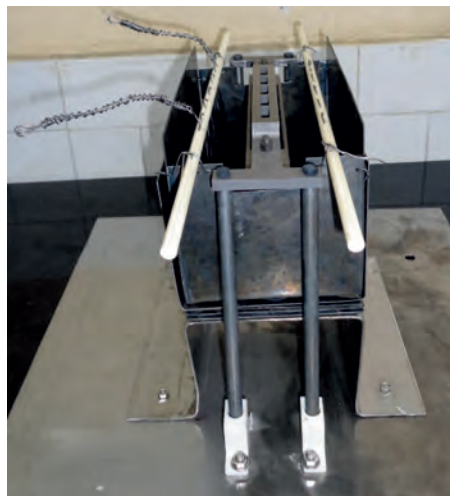
Figure 19.4: Photograph of a electron bombardment heating furnace used for generation of Lutetium (Lu) vapor.
