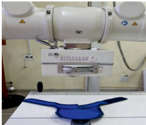
Figure 9 (a): Experimental set-up showing medical diagnostic x-ray machine and the apron to be tested for its lead equivalence.
