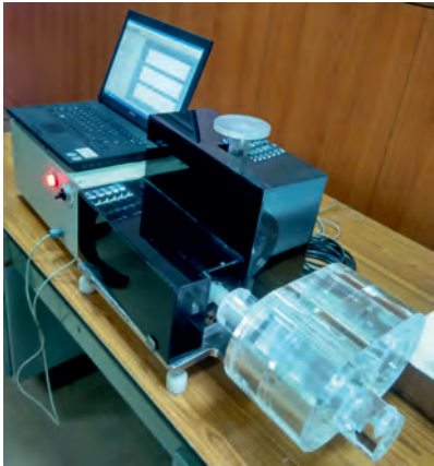
Figure 3(a): 4D dynamic phantom and its control system
