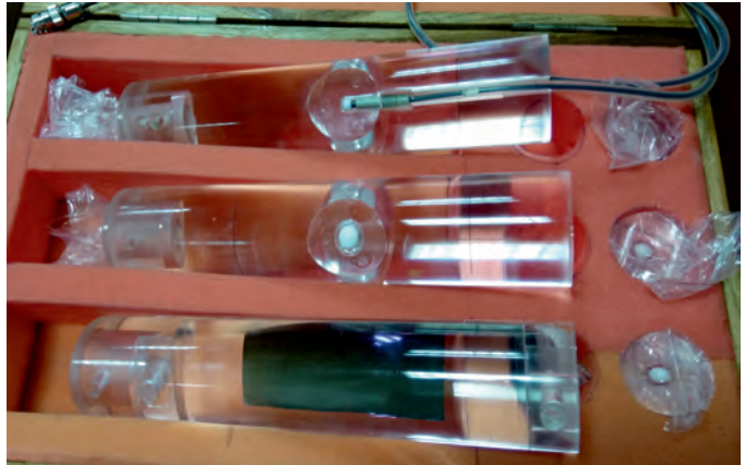
Figure 3(b): Replaceable lung-inserts representing PTV
