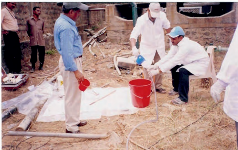
Figure 13: Groundwater velocity measurement
