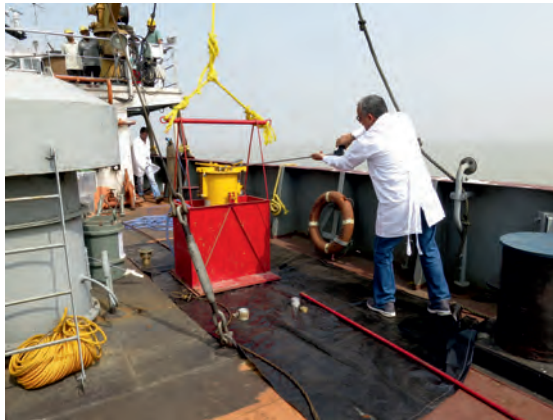
Figure 8: Injection of radiotracer for sediment transport
