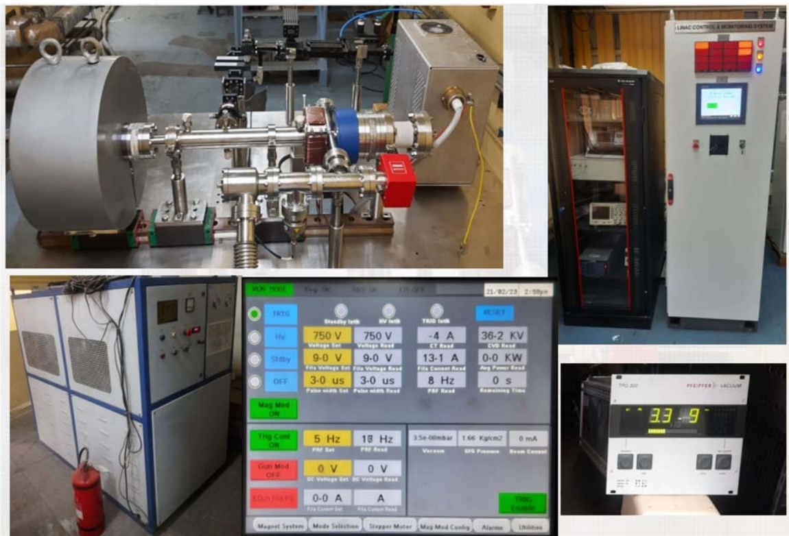
Compact 6 MV X-Band Linac and Auxiliaries
