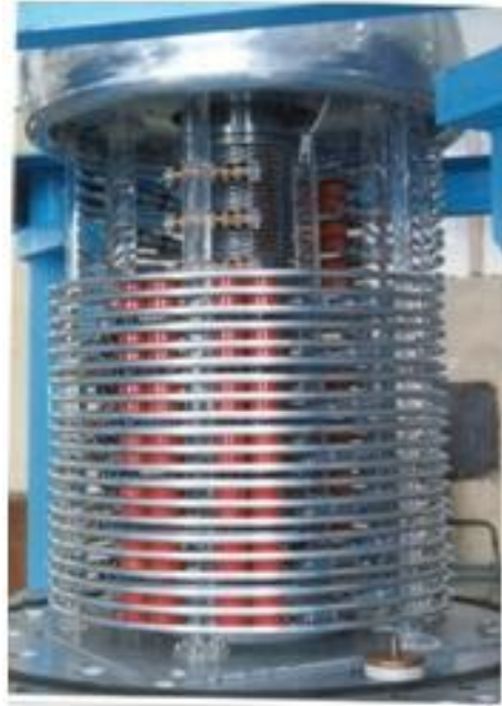
500keV Accelerator Multiplier Column
