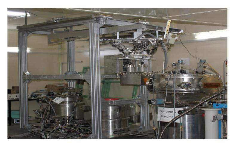
A 6 DOF Hexapod mounted on a telescopic X-X' table for alignment of mirror is developed and installed at beamline BL-8, RRCAT, Indore. The X-X' table is used to position the mirror chamber along with the beamline. The Hexapod can provide controlled motion for highly fine alignments both in position and orientation.
