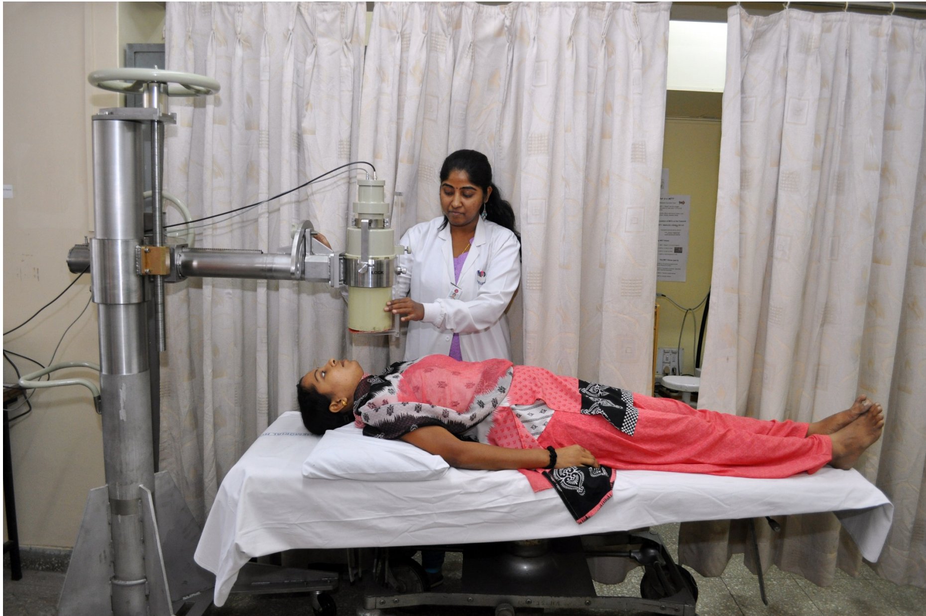
Fig: Manually Operated Thyroid Probe Manipulator Assembly
