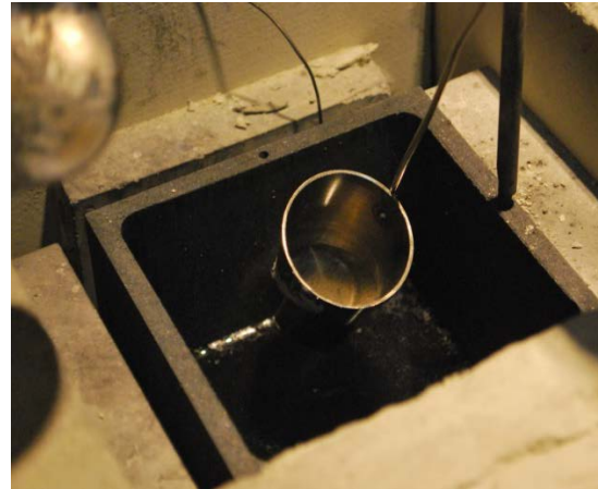
Graphite crucible containing molten fluoride salts
