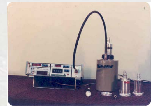
Scintillation counting set up of radon
