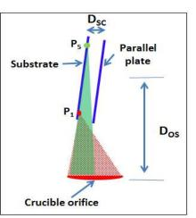
Glancing Angle Deposition (GLAD) of Silver films with angle constrainment using a parallel plate (Top)
