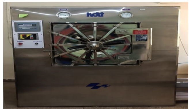
Fig.8: Single Door High-Pressure High-Vacuum (HPHV) semi-automatic rectangular autoclave: Sterilization of cages, water bottles, bedding material and disposable aprons.
