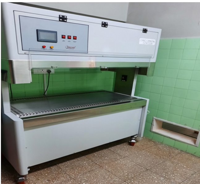
Fig.6: Animal cage change station: Daily routine use for cage changes in the rat and mice.
