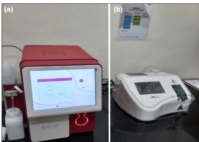
Fig.10: Veterinary Haematology and serum biochemistry analyzer: (a) Haematology Analyzer. (b) Serum Biochemistry analyzer.
