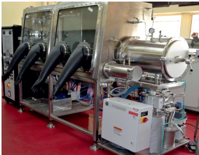
Fig.9: Glove box equipped with thermal evaporation system.
