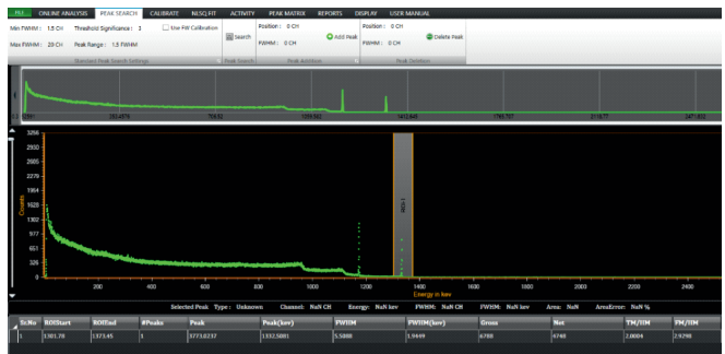
Fig.21: FWHM resolution of ~1.95 keV @ 1332.5 keV Co-60 peak.
