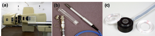
Fig.2: a) Tele-cobalt calibration facility, b) Typical cylindrical ionization chamber, c) Parallel plate ionization chamber.
