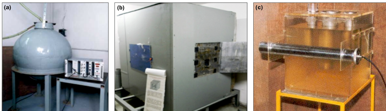
Fig.13: a) Manganese sulphate bath system, b) Thermal stag, c) Portable Thermal neutron water jig.
