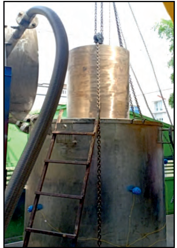
Fig.8 Loading of hull drum in furnace
