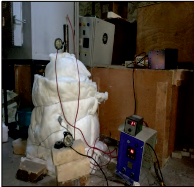
Fig.2 Experimental setup for Feasibility of hull drying using electrical resistance heating furnace
