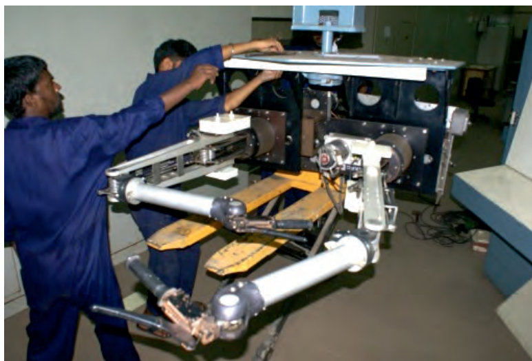
Master arm dismantling from swivel plate
