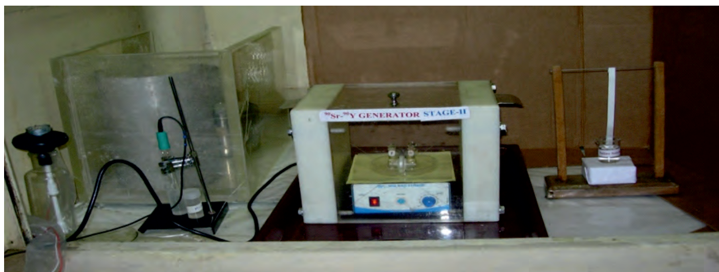
Fig.7: 90 Sr- 90 Y generator system housed in Fume-hood at PP
