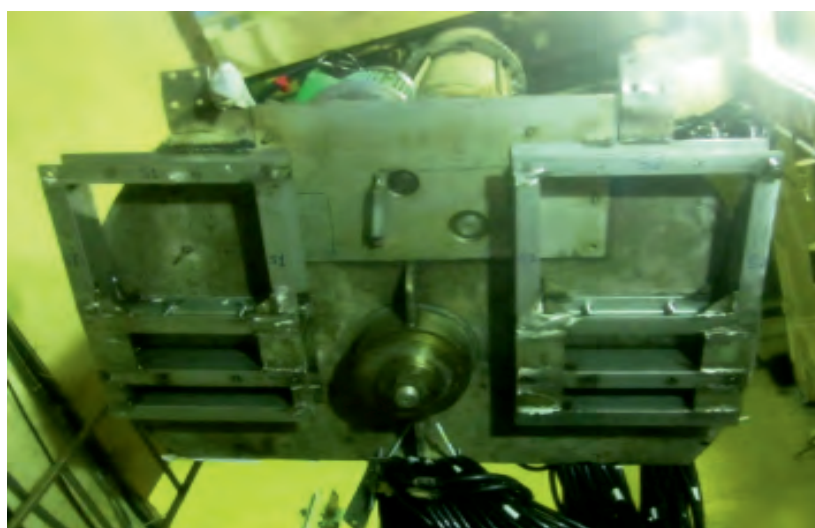
Figure 13. Bracket for re-orientation of Slave arm
