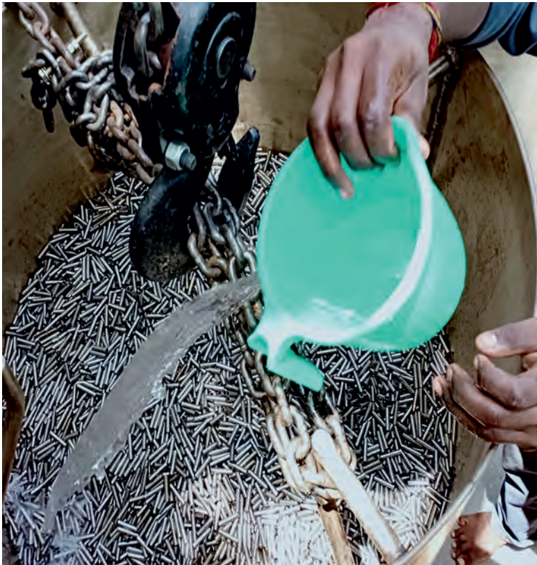
Fig.7 Addition of water in hull drum
