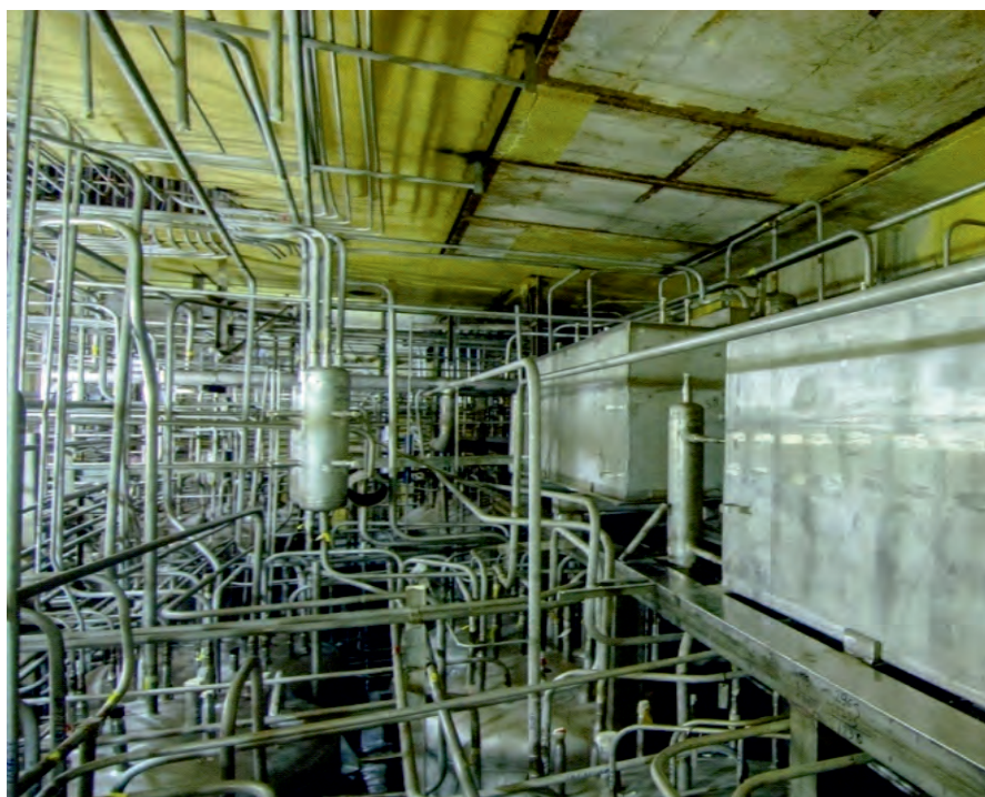
Fig. 1: Solvent extraction plant for separation of radionuclides from HLLW
