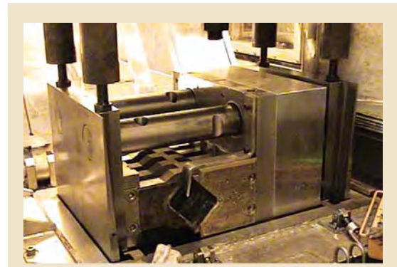
Fig. 7: Remote handling trial of shear module of SFC at ROP, Tarapur
