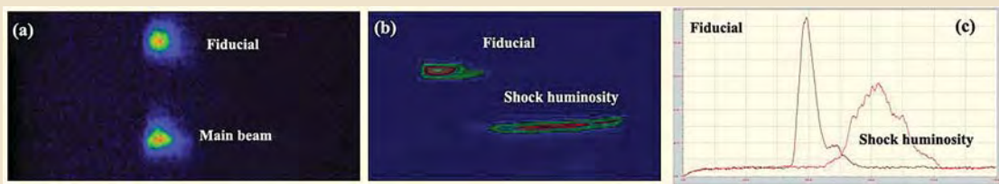
Fig. 2: Shock velocity measurement: (a) Synchronization of main beam with fiducial. (b) Streak record of the fiducial and shock luminosity signals in 10 μm Al foil at laser intensity 1 \times 10^{14} W/cm 2 (c) Plot of intensity profile of fiducial and shock luminosity. X-axis shows time in terms of pixel numbers (1 pixel = 6.56 ps) and Y axis shows intensity of the glow in numbers of pixels.
