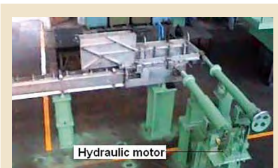
Fig. 3: Fuel feed system with hydraulic drive
