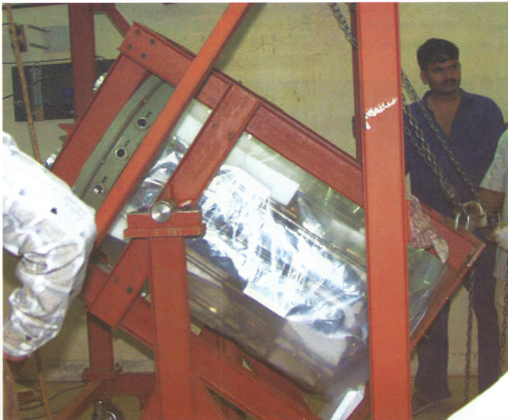
Fig. 5 : Internal structures with support frame being tilted with the help of base structure and pivot
