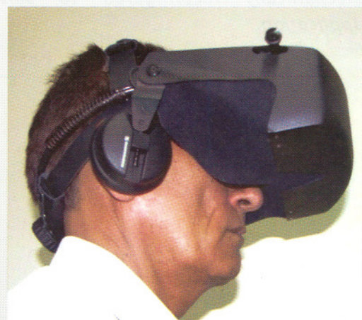
Head Mounted Display (HMD) for the stereo vision system (under development)
