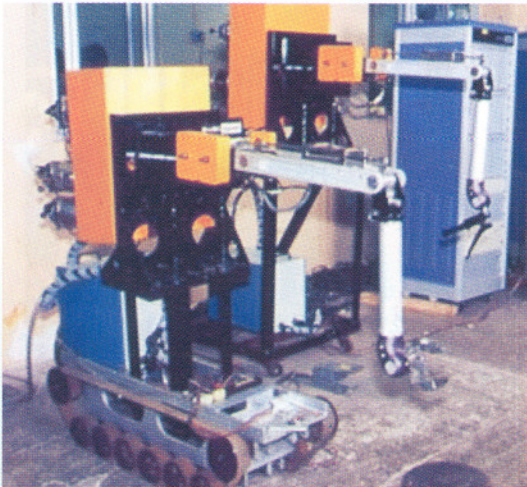
Indigenous servo manipulator: The slave arm is mounted on tracked vehicle
