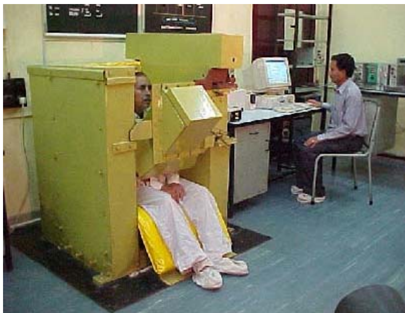
Fig. 1. Photograph showing the shielded chair whole body monitor. Mounted on the top right side is the electrical motor along with its gear and pulley mechanism.
