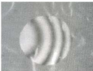
Curved fringes for a plane surface showing a peak error of \lambda/2.5 .
