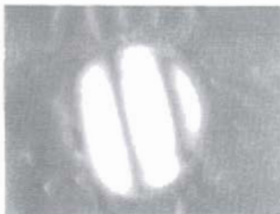
Straight, equally spaced fringes for a plane surface showing a peak error of \lambda/10 .
