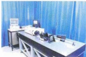
Fig. 4 Zygo phase measuring interferometer for precision testing of optical components
