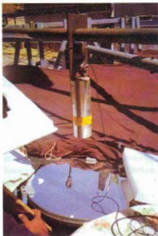
Fig. 5 Laser based Plumb Line positioned over a mirror
