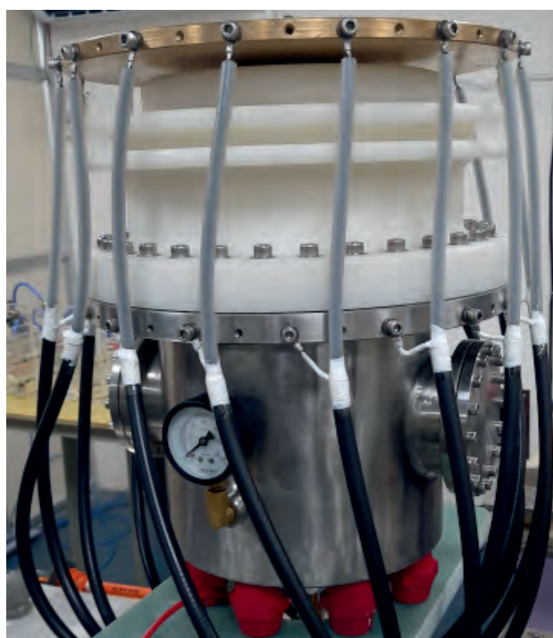
The Technology of High Coulomb Spark-gap Switch with Applications in Large Charge Transfers Associated with High-energy Pulsed Power Systems.
