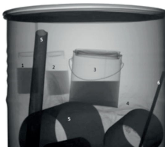
Image of a test drum generated using X-ray imaging system developed in BARC.
