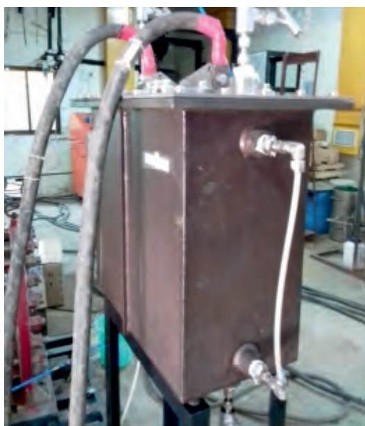
Tank-type electrolyzer assembly.
