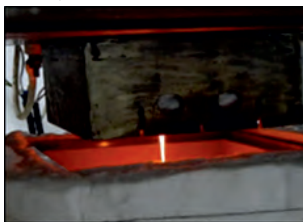
Casting trial of 200 x 200 glass slab of RSW.
