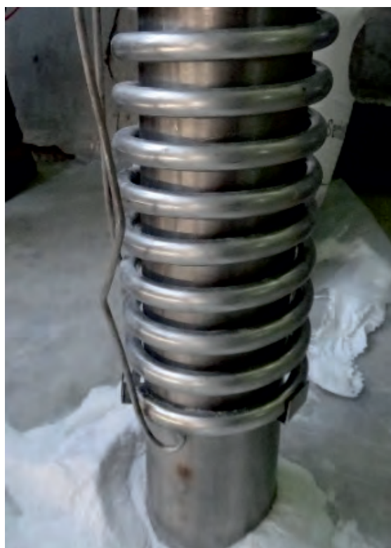
Coil-in-Coil type Recuperator of Cryogenic Purifier Modules.
