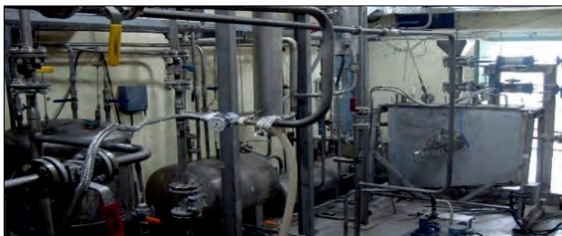
Test loop of continuous pellet dissolution facility.
