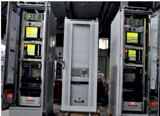
ESCADA panels undergoing burn-in test.
