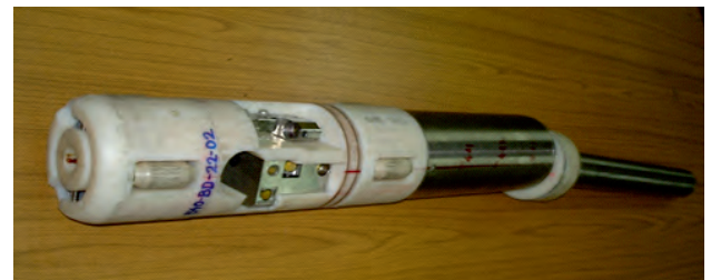
Inspection Head for 540 MWe PHWRs.
