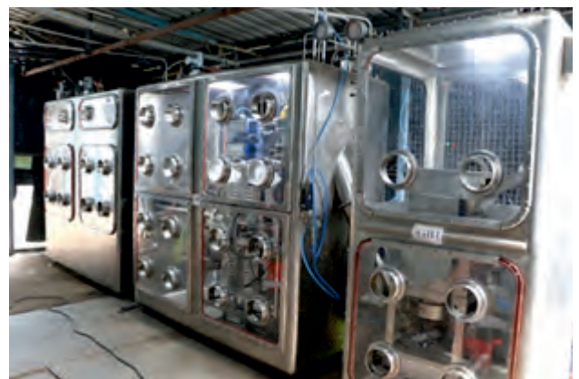
Glove Box demonstration setup for pyrolysis based polymeric and cellulosic waste treatment.
