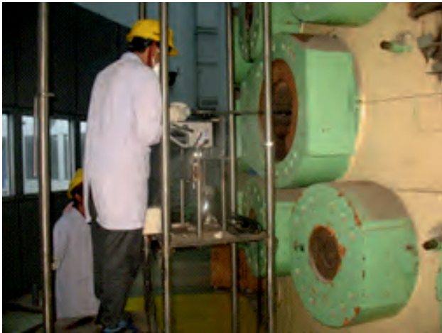
Remote System being aligned with neutron beam hole.
