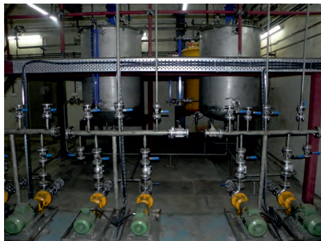
Pilot Plant for purification of slag leached solution (SLS).
