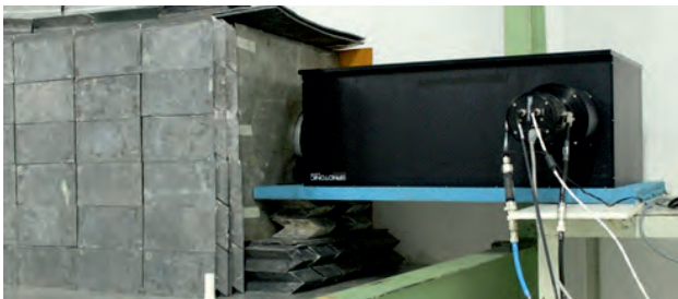
Neutron radiography set-up with gated ICCD camera for imaging.
