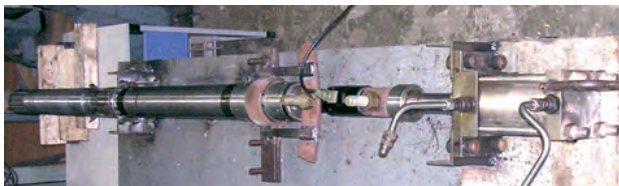
Setup for pull-test of Wet Quarantine Plug.
