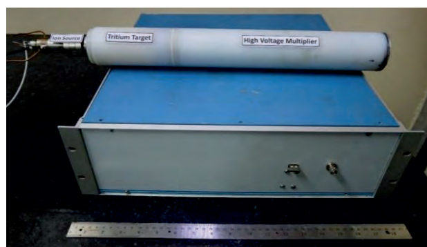
A sealed 14 MeV D-T neutron source along with its control unit.
