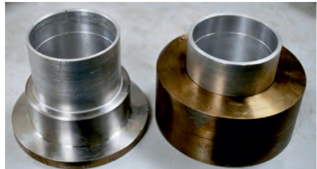
Diffusion bonded joint (SS 304 to Aluminium 6061).
