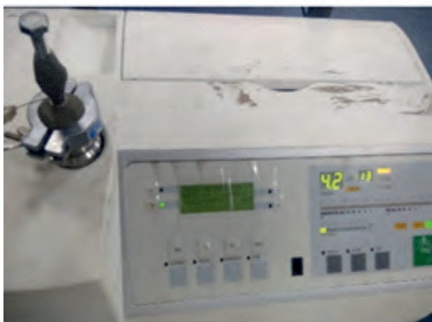
Helium leak rate measurement.
