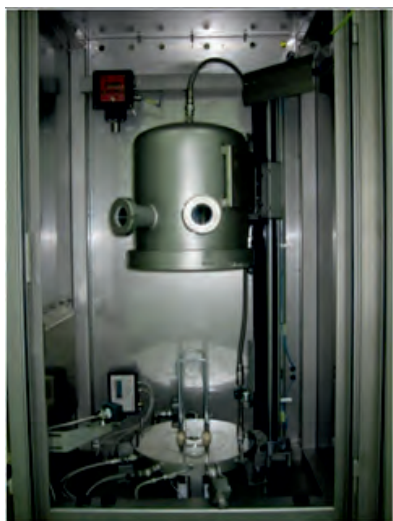
CVD reactor for production of high purity Silicon.
