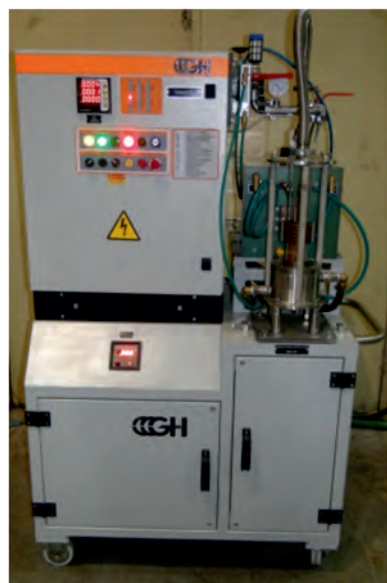
Induction Levitation Melter.
