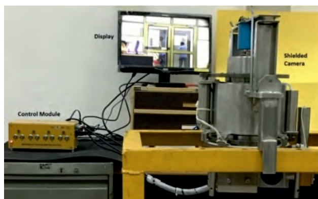
Shielded camera and its control system.
