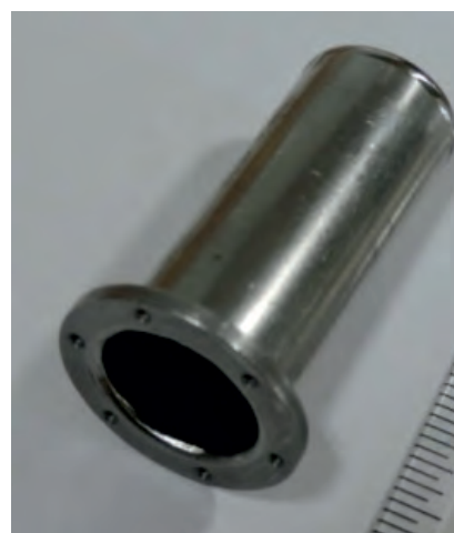
Niobium cans welded using Electron Beam Welding machine.
