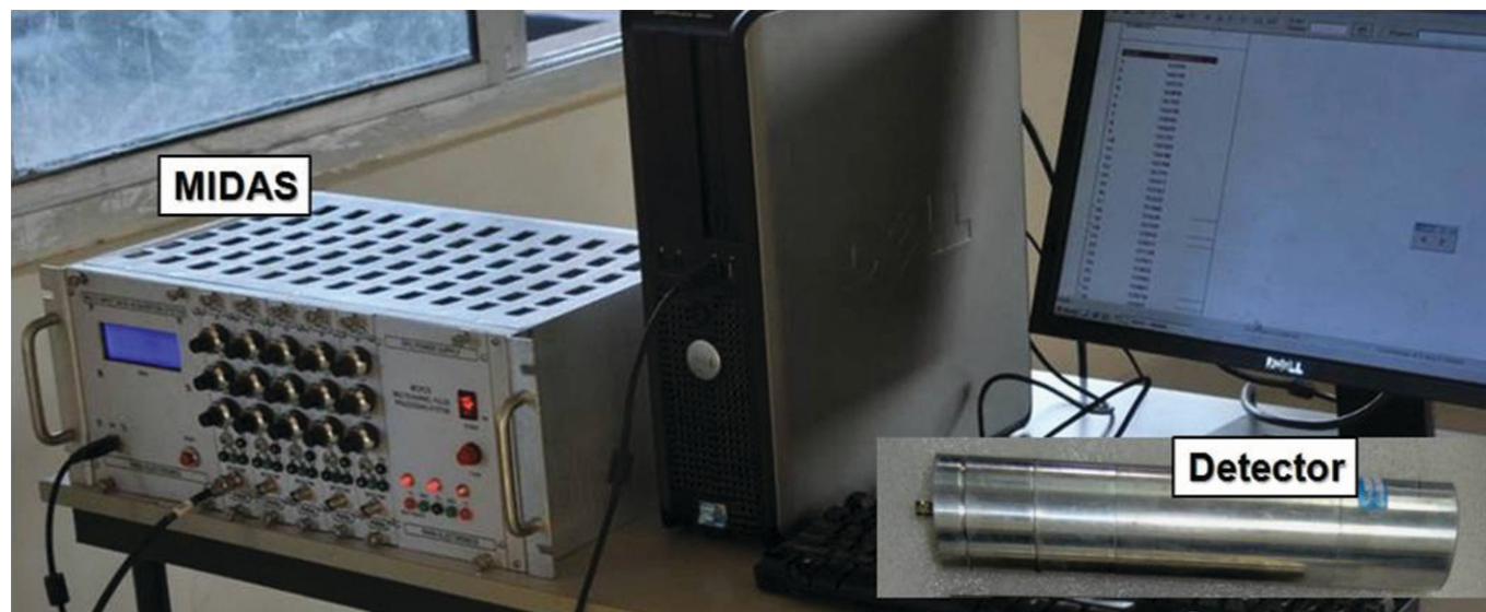
Fig. 7. Multi-input data acquisition system (MIDAS) with a NaI(Tl) scintillation detector
