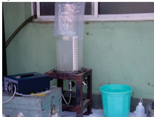
Fig. 4: Injection of radiotracer into suction end of the CV pump
