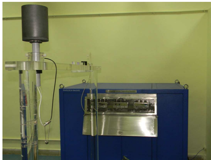
Fig. 6: Photograph of the experimental set up used for measuring the strength of HDR ^{192}\text{Ir} brachytherapy source stored in the multisource remote operating device. Large volume graphite ionization chamber and PMMA source calibration jig can also be seen in this photograph
