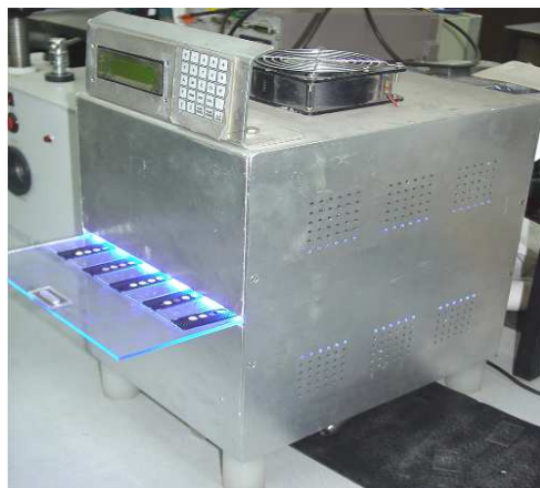
Fig. 9: Optical bleaching setup for resetting the OSLD badges
