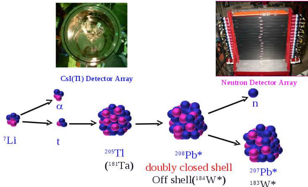
Fig. 2: Schematic of the reaction mechanism used to populate the nuclei of interest to address the damping of nuclear shell effect and the detector array used for the charged particle and neutron measurement
