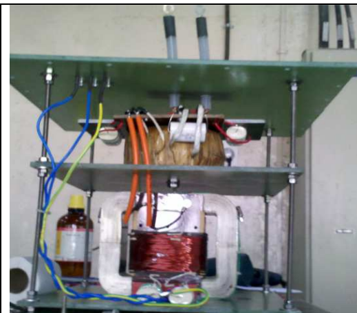
Fig. 3: 1:5 HV Pulse Transformer
