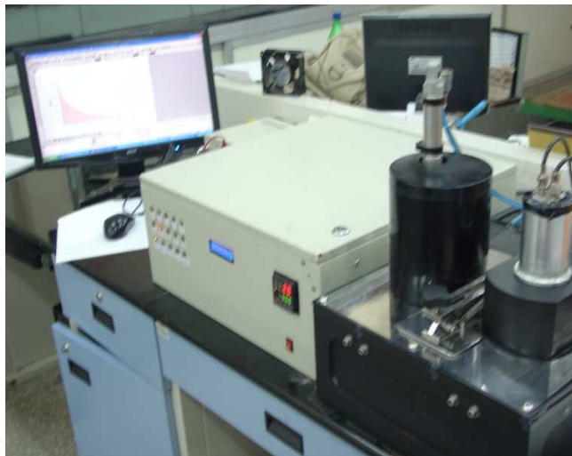
Fig. 12: Multi sample integrated TL-OSL Reader system for luminescence dating and research applications
