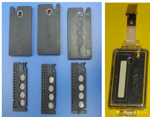
Fig. 6: Prototype four element OSLD badge. (a) Plastic dosimeter card having built-in machine readable ID code which contains thin \text{Al}_2\text{O}_3:\text{C} OSL dosimeters and light-tight black cassette to house the plastic dosimeter card (b) OSLD badge with transparent plastic cover
