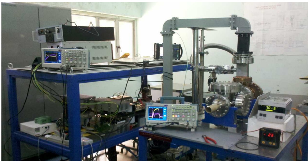
Fig. 9: Modulator used for powering the e2v make magnetron MG5028 used for buncher Linac Conditioning
