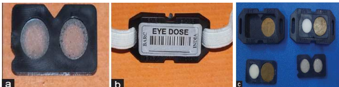
Fig. 4: (a) Two element \alpha -Al 2 O 3 :C dosimeter card, (b) eye lens dosimeter badge & (c) Proposed eye lens dosimetry badge showing the two element OSL card along with plastic cassette and energy compensating filters
