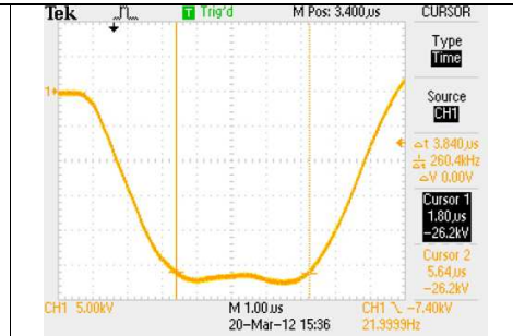
Fig. 13: 53kV Pulse across the electron gun
