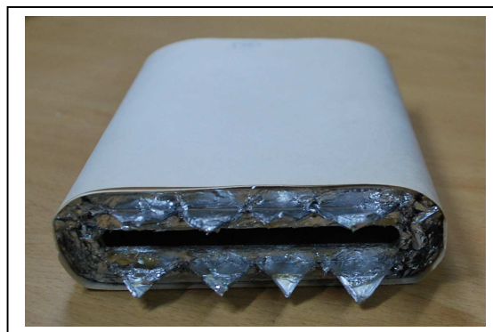
Fig. 1: Flat format pulse capacitor 4 \mu F, 5.5kV
