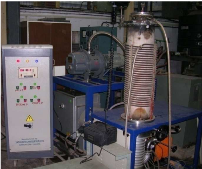
Fig. 2: Induction furnace for synthesis of powders carbide
