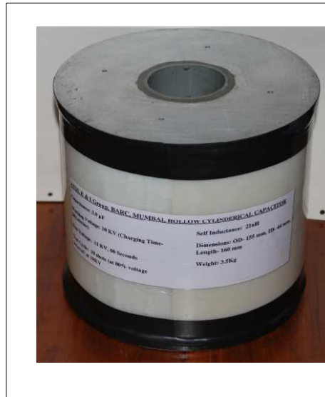
Fig. 2: Hollow cylindrical pulse capacitor 10kV
