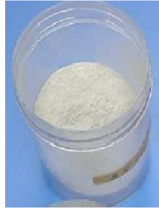
Fig.2(b): Al 2 O 3 :C powder on pulverisation
