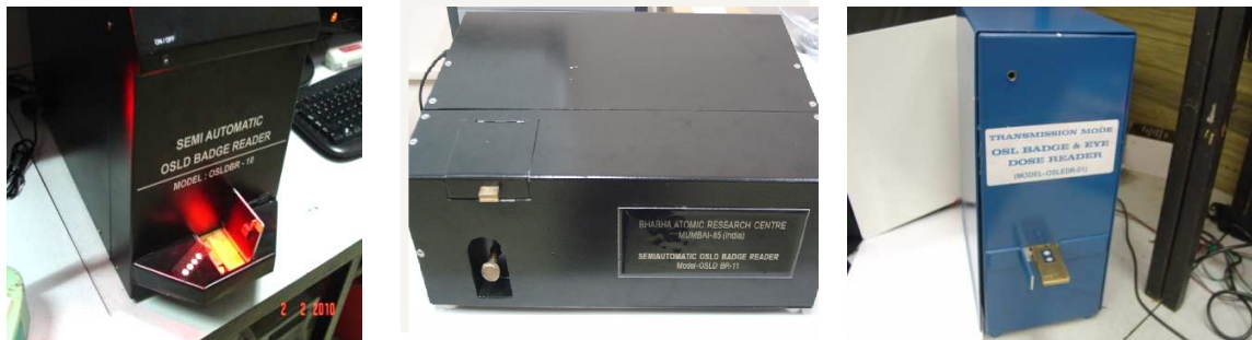
Fig. 7: Reflection and Transmission mode Semiautomatic OSLD badge reader systems
