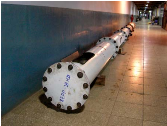
Fig. 3a: 10 m Long Pipe Assembly
