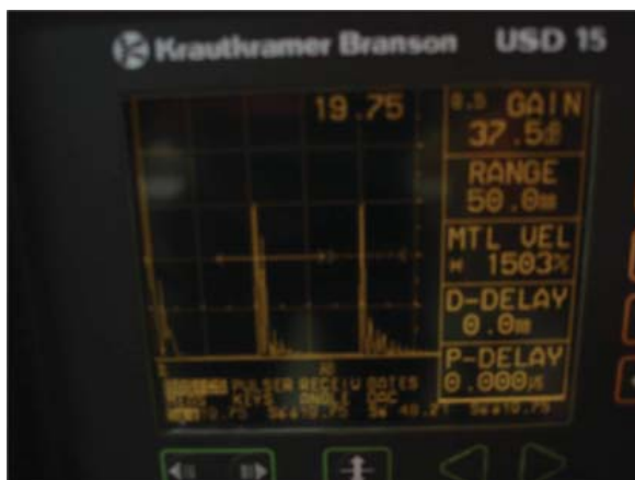
Fig.3: Water Path Measurement by Ultrasonic Probe
