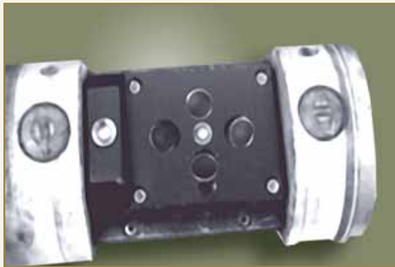
Fig. 2: Inspection head for pressure tube examination
