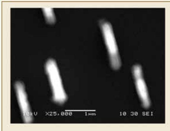
Fig. 3: SEM micrograph of 60 Å Cu film deposited on Si(110) at 750°C
