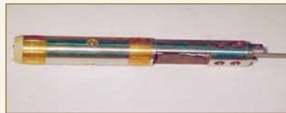
Fig. 3: Inspection head for ID measurement system
