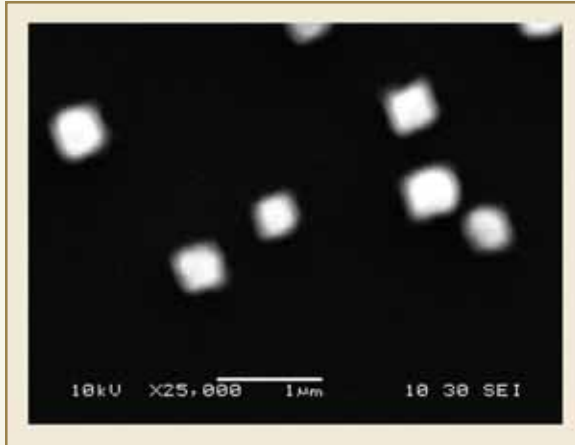
Fig. 2: SEM micrograph of 60 Å Cu film deposited on Si(100) at 750°C
