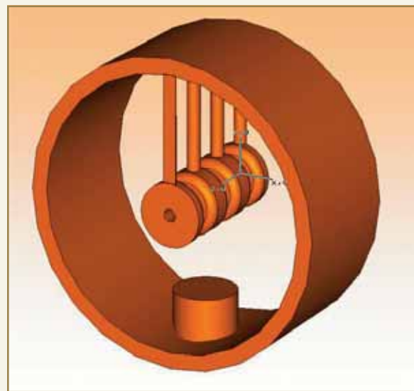
Fig. 5: A 3-cell model of a DTL cavity with tuner
