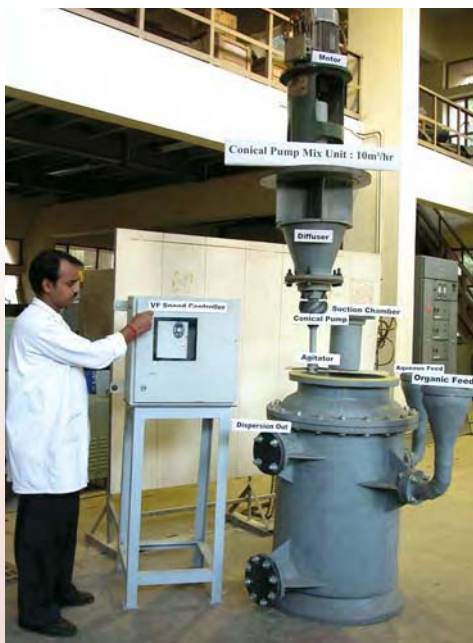
Fig. 4: Photograph of internal details of a pump mix unit
