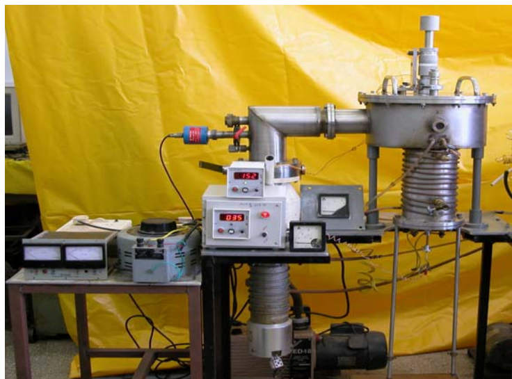
Fig. 7c PIA experimental setup for I and Te release studies
