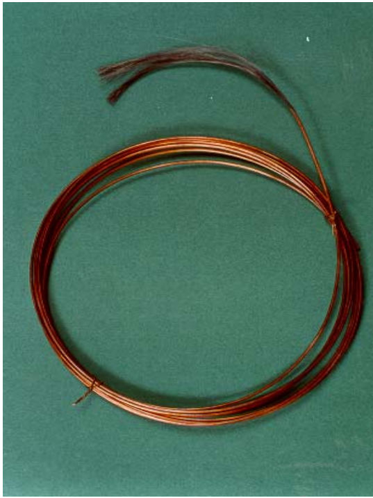
Fig.3 1.3mm dia Cu/Nb/Nb-Ti superconducting wire (492 filaments, 40 micron size)
