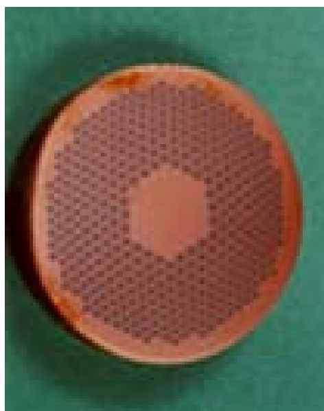
Fig.2 Cross section of extruded Cu/Nb/Nb-Ti rod (50mm dia)
