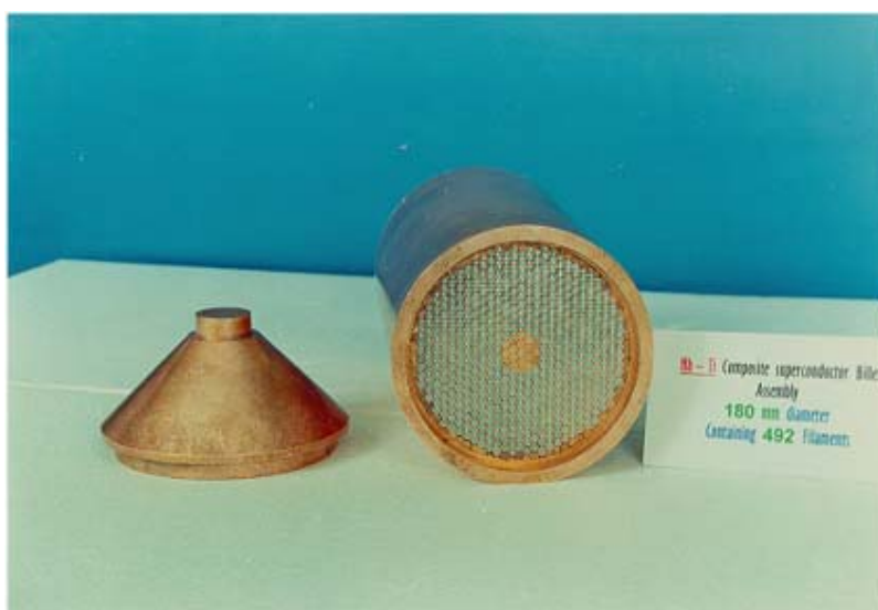
Fig.1 Cu/Nb/Nb-Ti multifilamentary billet assembly developed at AFD
