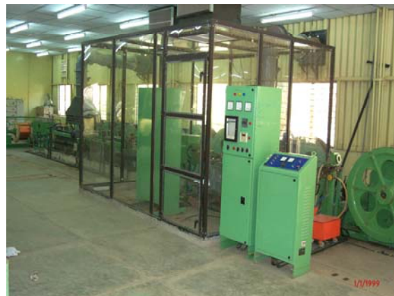
Fig.6 Continuous soldering unit for superconductor wire
