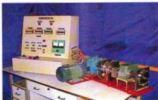
Test rig for qualification of spiral spring, rotary switchgear and potentiometer
