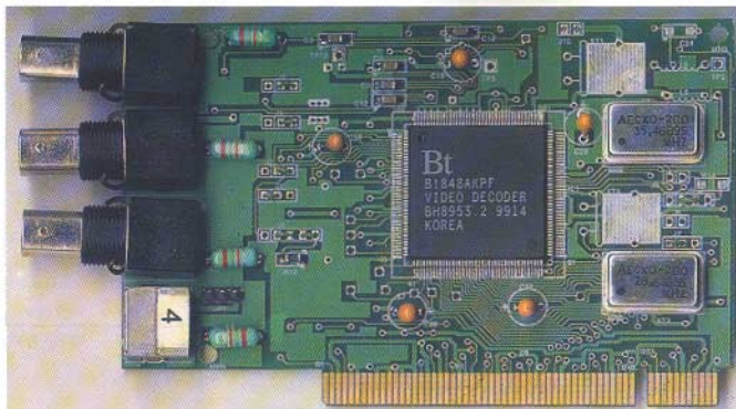
Fig. 4 PCI bus based video image capture card.
